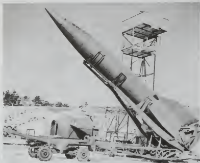
Figure 20: German V-2 missile being erected for launch. This "Vengeance Weapon" of World War II, which struck cities 200 miles away, was the precursor of modern ballistic missiles.
